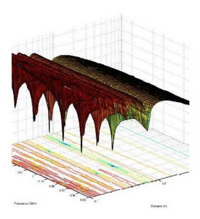
Figure: Path loss over a flat reflecting surface.
